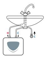
Do not install upside down. Installation must conform to sans 10254
